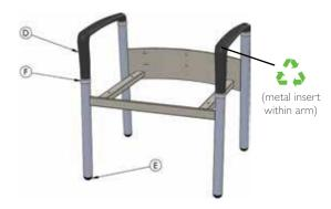
**D & E:** Place the chair on its side. Using firm blows with the hammer, knock the polyurethane arm free out of the frame. Remove the aluminum transition rings. Next, take the flat blade screwdriver and hammer pry the glides free from two of the legs. Flip the chair over and repeat the process for the other side.
