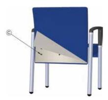
**C**: Using the #2 Philips screwdriver, remove the six screws securing the back.
