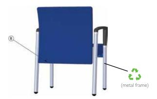
**B:** Set the chair upright. Standing behind the chair pull down on the bottom edge of the upholstery and unclip the J extrusion from the back bar. Pulling up the fabric will expose the screws securing the chair back to the chair frame.
